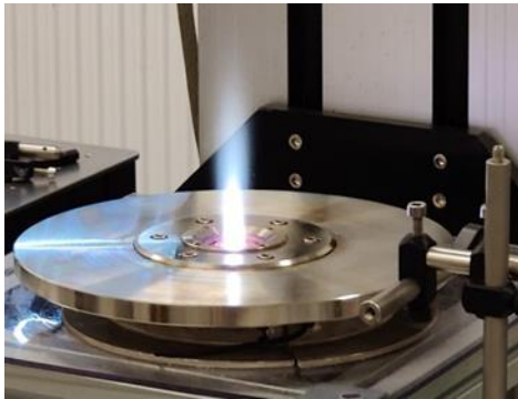
Figure 3: The plasma jet (or flame) from a laboratory plasma burner (Swerim)
