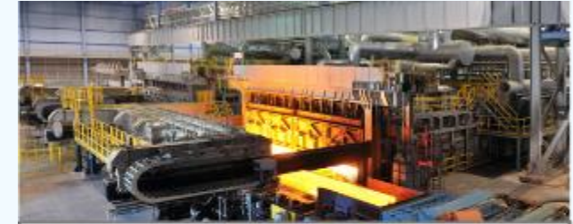
Walking Beam Furnace 300 tph Slab discharging temperature: 1250 °C Specific NG consumption: 1.3 GJ/ton
